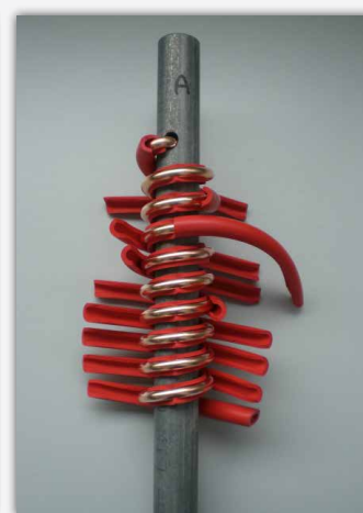
Stress bending test at high temperature with standard compound
