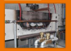
This test is carried out to verify the circuit integrity of cables exposed to fire at 830°C and mechanical shocks. During the tests the cables are maintained at their rated voltage.
