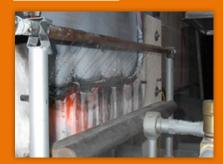
This test is carried out to verify circuit integrity during a fire. The cable is exposed to a flame at 930°C and mechanical shocks for 60 minutes and additional 60 minutes to flame, mechanical shocks and water spray. During the tests the cables are maintained at their rated voltage.
