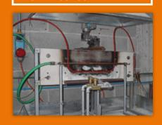
fire. The cable is exposed to a flame at 830°C and mechanical shocks for 15 minutes and additional 15 minutes to flame, cables are maintained at their
